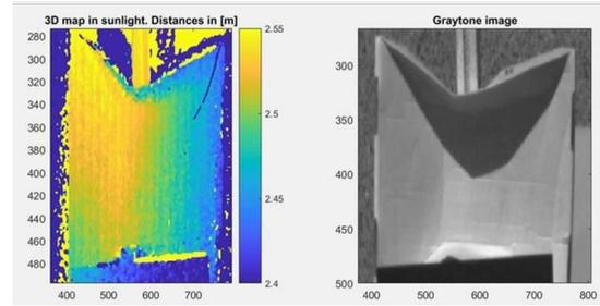
Figure 6: Example of Structured Light 3D map
