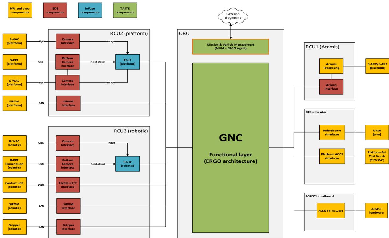
Figure 10: EROSS SW architecture
