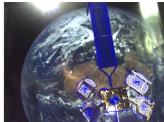
Figure 7: Example of ARAMIS 3D pose estimation
